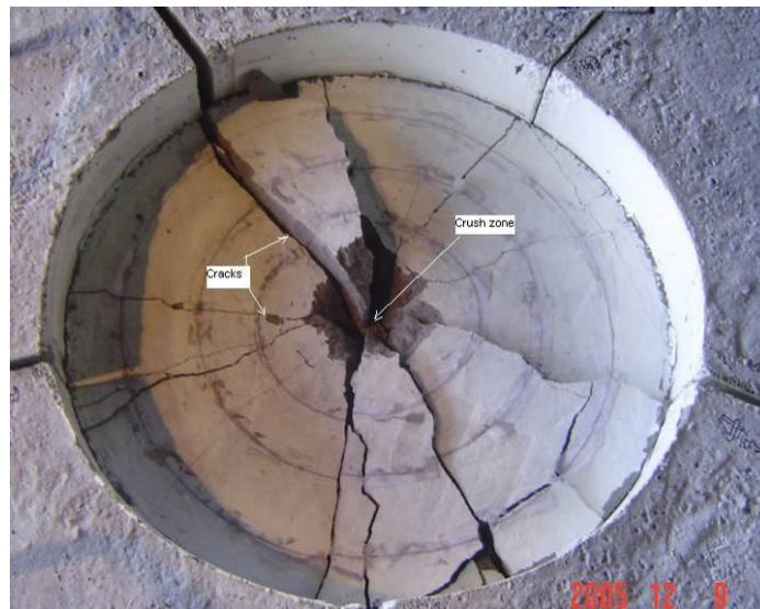
Figure 10.20. Postblast grout sample #6 fully-coupled explosive 207X and confined
