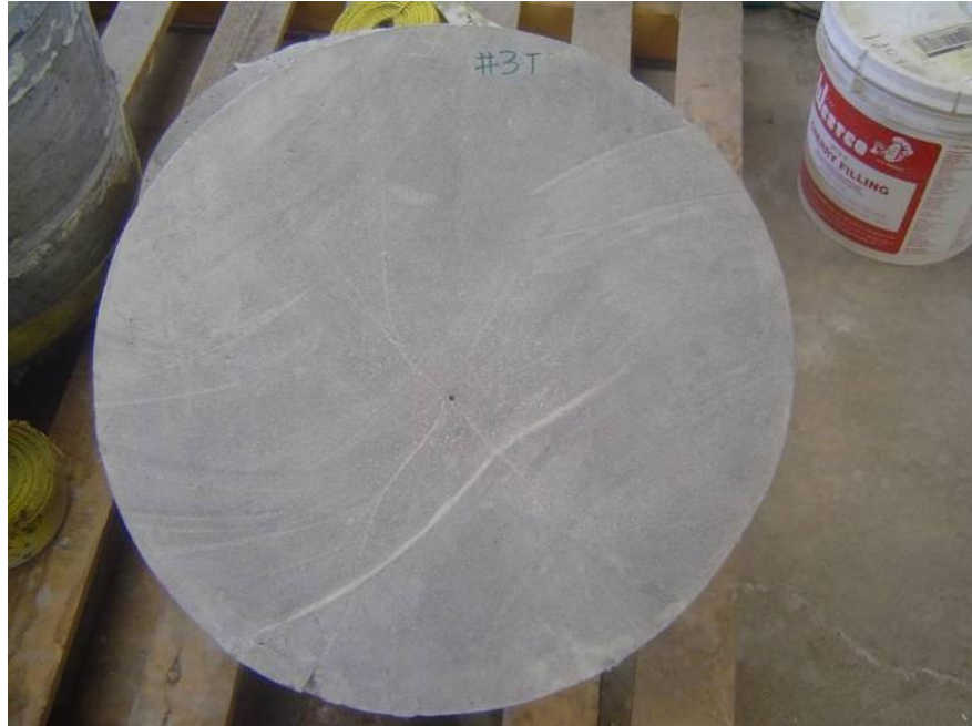
Figure 10.14. Postblast sample #3, 3.6 gram/m detonating cord, fully-coupled and confined
